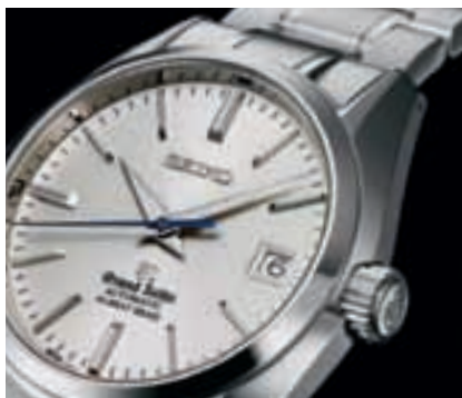
SEIKO GRAND SEIKO 50 TH ANNIVERSARY. FIVE YEARS IN DEVELOPMENT, THE SELF-WINDING CALIBER 9S85 BEATS AT 36,000 VIBRATIONS PER HOUR. THE BALANCE SPRING DELIVERS AN EXTENDED 55-HOUR POWER RESERVE WITH NO LOSS OF PRECISION. SAPPHIRE CRYSTAL CASEBACK. WATER-RESISTANT TO 100 M.
