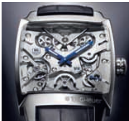
TAG HEUER MONACO V4. THE UNIQUE BELT-DRIVEN SELF-WINDING MECHANICAL MOVEMENT BUILDS ON ENGINE TECHNOLOGY. THE OPEN DIAL REVEALS THE MECHANISM WITH HAND-FINISHED BRIDGES. BLUE FACETTED HANDS, SMALL SECONDS AT 4 O'CLOCK. EXCLUSIVE TUNGSTEN LINEAR OSCILLATING WEIGHT CONNECTED TO TWO PAIRS OF COUPLED BARRELS WITH DIFFERENTIAL LINK. 40.5 MM SQUARE PLATINUM CASE. WATER-RESISTANT TO 50 M. ALLIGATOR STRAP WITH BLUE TOP STITCHING. LIMITED EDITION OF 150.
