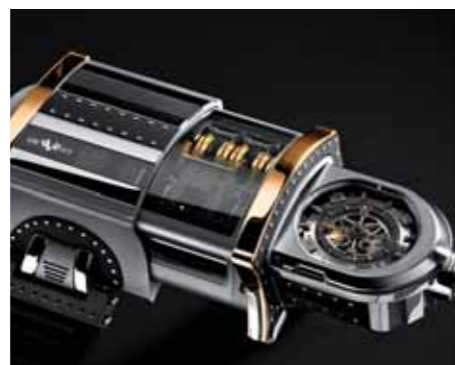
DEWITT WX-1 . AN AUTHENTIC MACHINE, THE PULSATING HEART OF THE WX-1 IS EQUIPPED WITH A VERTICAL FLYING TOURBILLON WITH A CARRIAGE PERFORMING ONE REVOLUTION PER MINUTE AND VISIBLE THROUGH A CYLINDRICAL "CHIMNEY" LOCATED ON THE BACK OF THE CASE. THE MECHANICAL HAND-WOUND MOVEMENT COMPRISES A PARALLEL GOING TRAIN WITH FIVE BARRELS ENSURING A 21-DAY (APPROXIMATELY 504-HOUR) POWER RESERVE. THE PARTS MAKING UP THIS "COMPETITIVE RACING" ENGINE — BARRELS, GEAR TRAIN, TOURBILLON CARRIAGE, POWER-RESERVE INDICATOR AND WINDING DEVICE — ARE ALL ARRANGED IN VERTICAL ORDER. THE POWER RESERVE IS DISPLAYED BY A COAXIAL ROLLER, WHILE THE TIME OF DAY IS READ ON TWO ROTATING DISCS. THE FIRST, SHOWING THE MINUTES, TURNS IN A CLOCKWISE DIRECTION, WHILE THE ONE DISPLAYING THE HOURS TURNS COUNTER-CLOCKWISE BY MEANS OF A CLEVER GEAR SYSTEM MOUNTED ON SIX RUNNERS.
