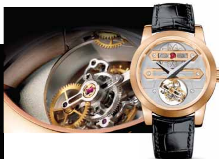
GIRARD-PERREGAUX BI-AXIAL TOURBILLON. THE BI-AXIAL TOURBILLON, COMBINING TWO CONCENTRIC CAGES, ENABLES THE REGULATING PART TO MAKE MULTI-DIMENSIONAL ROTATIONS. AN INTERNAL CAGE BEARING THE BALANCE, BALANCE SPRING, AND ESCAPEMENT COMPLETES ONE COMPLETE TURN ON ITS AXIS IN FORTY-FIVE SECONDS. AN EXTERNAL CAGE COMPLETES ONE REVOLUTION IN ONE MINUTE AND FIFTEEN SECONDS, ENABLING A ROTATION ON ITS SECOND AXIS. A FULL REVOLUTION IS COMPLETED IN THREE MINUTES AND FORTY-FIVE SECONDS. THIS GENUINE AERIAL BALLET OFFERS AN EXTRAORDINARY SPECTACLE, WHILE THE ALTERNATION OF POSITIONS ENABLES EXCELLENT RATE PRECISION.
